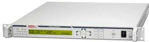
WORK Microwave's high-speed DVB-S2 IP modem SK-IP provides operators with a platform for transferring IP/Ethernet data over DVB-S2 satellite connections. Ethernet frames and IP packets are encapsulated directly within DVB-S2 baseband frames, resulting in low encapsulation overhead.
