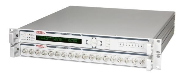
The WORK Microwave Redundancy Switch RSCC-8 is a compact solution for an 8:1 redundancy system. It can be used for Upconverters and Downconverters. The system consists of the controller and an indoor switch matrix integrated in separate 19" 1 RU housing.
