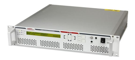
The A-Series is a next generation FPGA-based family of satellite modem, modulator and demodulator platforms. The AX-80 product line is based on a powerful architecture that supports the new DVB-S2X standard for ultra-wideband transponders up to 500 Msps. DVB-S2X features include higher modulation schemes up to 256APSK, a finer granularity of ModCods and advanced filtering.
