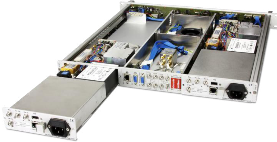
1+1 Redundant Block Converter System (cover not shown)
