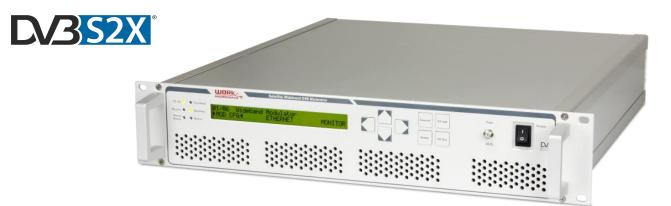
WORK Microwave's Wideband Modulator provides operators a platform for transferring Transport Streams in DVB-S2 multicast format as well IP/Ethernet data over DVB-S2/DVB-S2X satellite connections. Ethernet frames and IP packets are encapsulated directly within DVB-S2 baseband frames, resulting in low encapsulation overhead. For maximum bandwidth efficiency and ease of operation the device uses Generic Stream Encapsulation according to TS 102 606.
